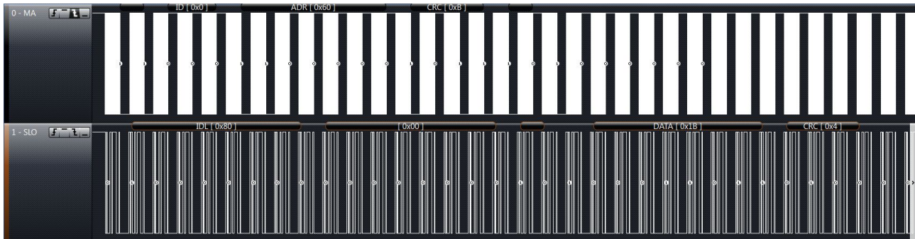
Figure 12: BiSS control communication for register access
