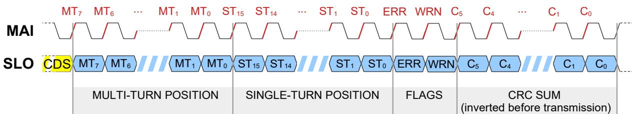
Figure 15: Typical Data Channel content
