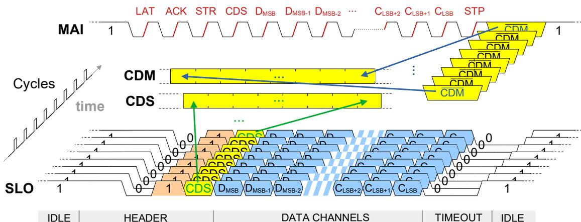
Figure 24: Multiple CDM and CDS bits compose the control data frame
