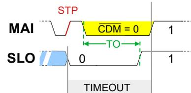
Figure 9: The Timeout of a simple *BiSS* frame
