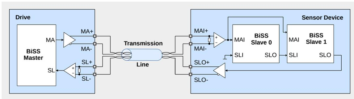
Figure 5: RS422 in point-to-point connection
