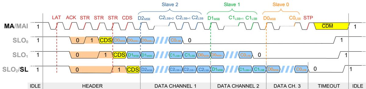
Figure 21: An entire *BiSS* frame passing through the daisy chain
