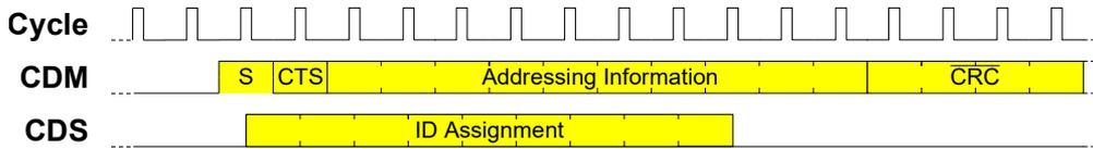
Figure 25: Header of the control data frame
