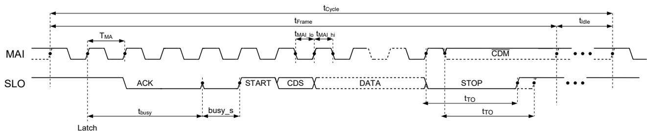
Figure 43: *BiSS* slave timings for point-to-point configuration
