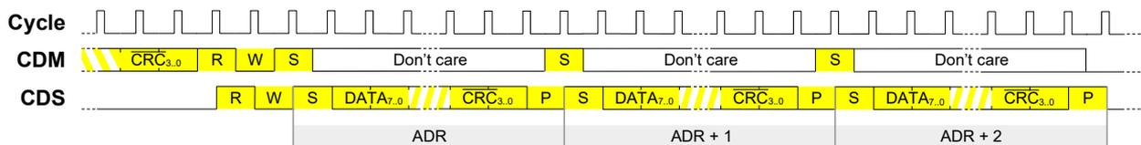
Figure 30: Register communication for sequential read access
