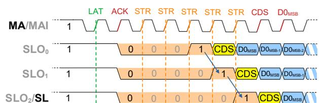
Figure 20: Start bit delay of daisy-chained *BiSS* Slaves
