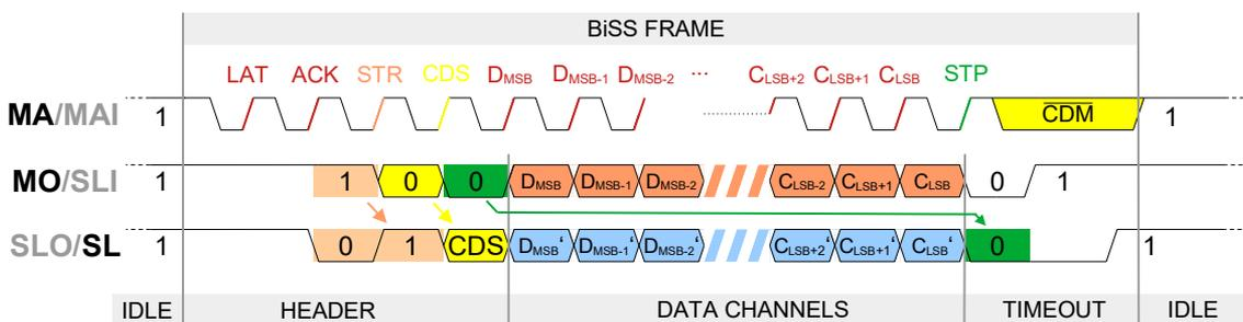
Figure 38: *BiSS* frame of single actuator bus system
