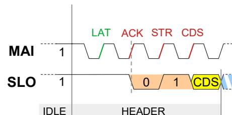
Figure 7: The Header of a simple *BiSS* frame
