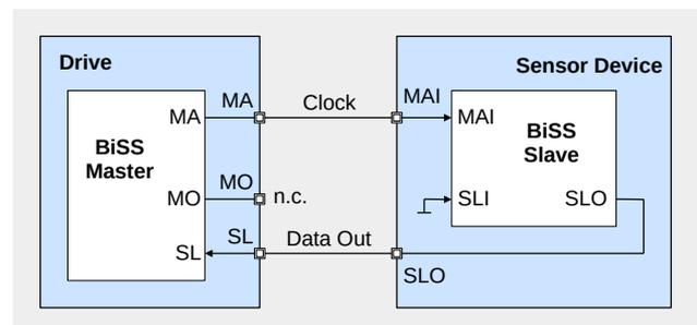
Figure 3: Point-to-point connection with a single *BiSS* Slave
