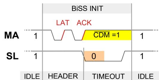
Figure 22: Example for a typical initialization sequence
