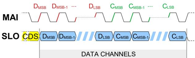
Figure 8: The Data Channels of a simple *BiSS* frame
