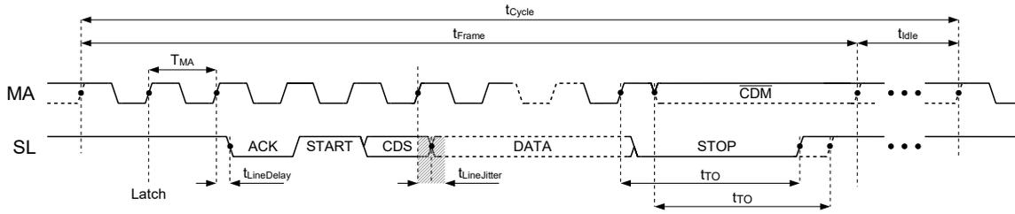
Figure 44: *BiSS* master timings for point-to-point configuration
