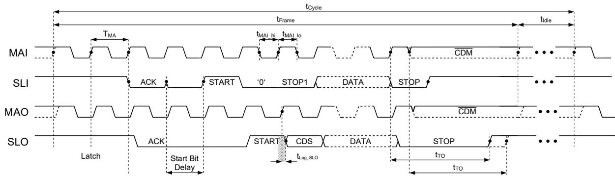
Figure 45: *BiSS* slave timings for bus configuration
