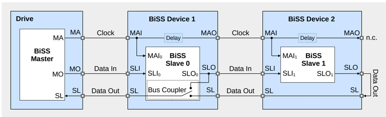
Figure 42: Bus Coupler in Device 1
