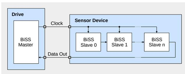
Figure 1: Point-to-point connection: master device connected to single sensor device
