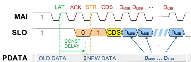
Figure 16: Constant delay of data generation
