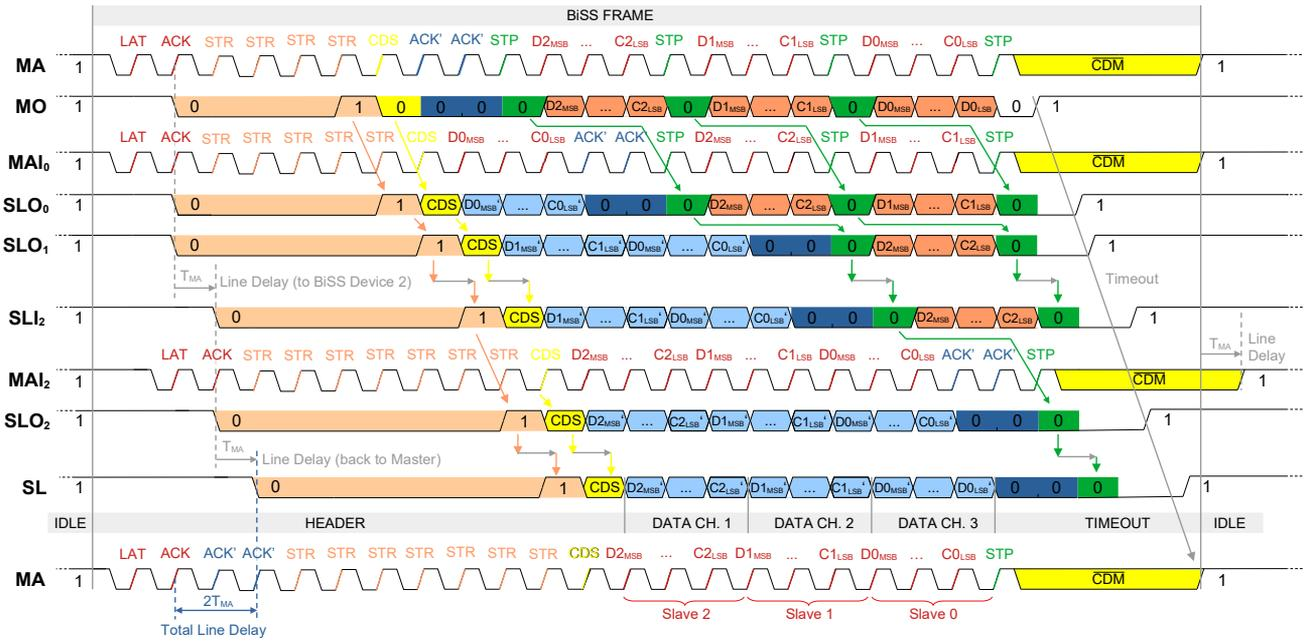
Figure 40: *BiSS* frame for daisy chain in bus connection with processing time
