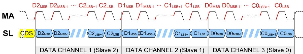
Figure 19: Data Channels of daisy-chained *BiSS* Slaves
