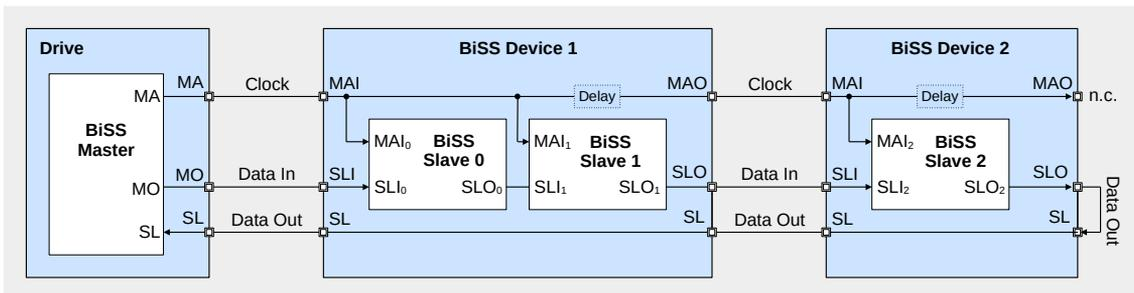
Figure 39: Daisy chain in bus connection
