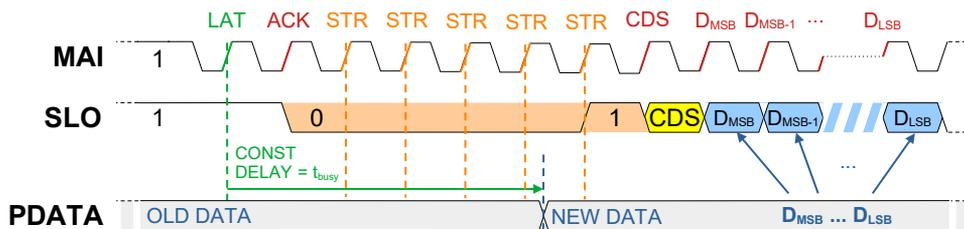
Figure 17: Delayed *BiSS* frame with significant processing time
