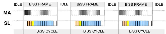
Figure 14: Isochronous *BiSS* cycles
