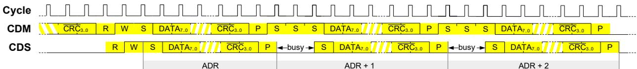
Figure 32: Register communication for sequential write access with start bit delay
