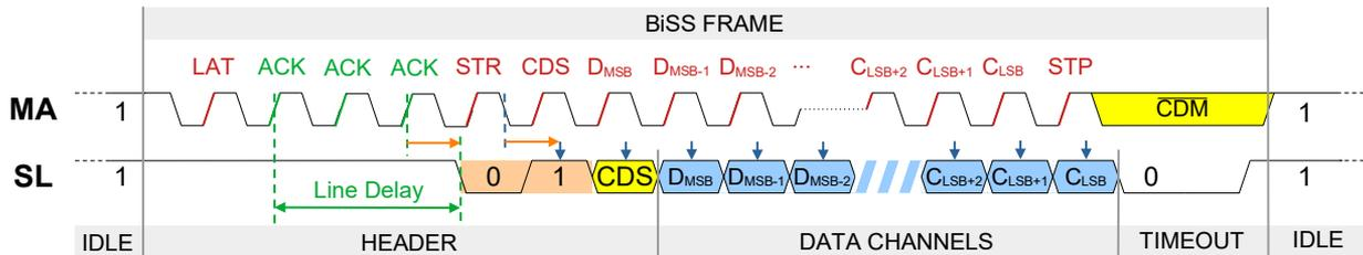
Figure 13: A *BiSS* frame with line delay at the *BiSS* Master
