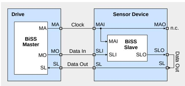
Figure 37: Bus connection with a single actuator slave
