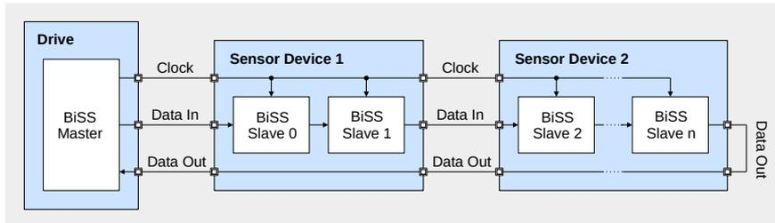
Figure 2: Bus connection: master device connected to several daisy-chained sensor devices
