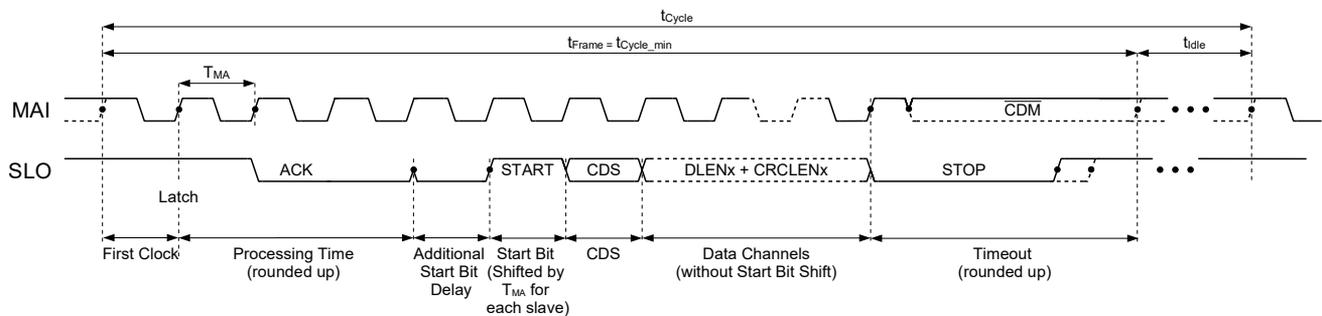
Figure 41: *BiSS* frame composition for calculation of minimum cycle time (line delay excluded)
