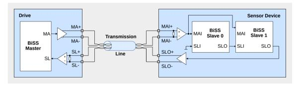
Figure 5: RS422 in point-to-point connection
