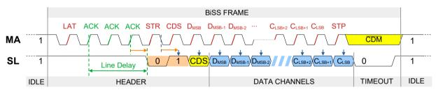
Figure 13: A BiSS frame with line delay at the BiSS Master
