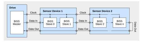
Figure 2: Bus connection: master device connected to several daisy-chained sensor devices
