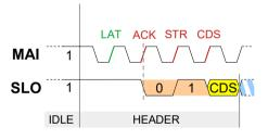
Figure 7: The Header of a simple BiSS frame
