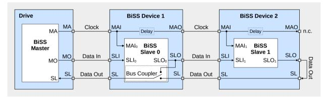
Figure 42: Bus Coupler in Device 1
