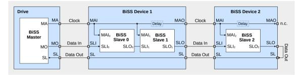
Figure 39: Daisy chain in bus connection
