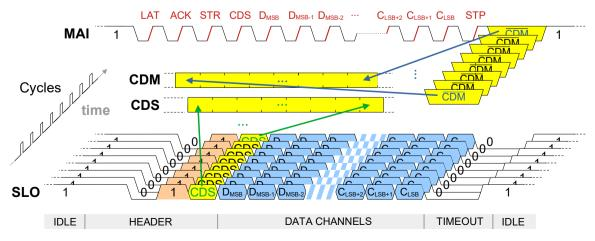
Figure 24: Multiple CDM and CDS bits compose the control data frame
