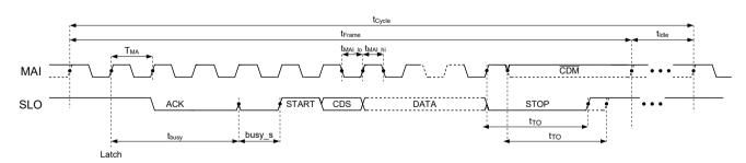
Figure 43: BiSS slave timings for point-to-point configuration
