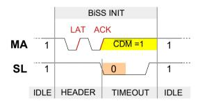
Figure 22: Example for a typical initialization sequence
