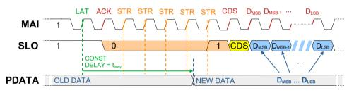
Figure 17: Delayed BiSS frame with significant processing time
