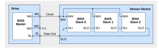
Figure 18: Daisy chain within a BiSS Slave device in point-to-point connection
