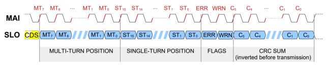
Figure 15: Typical Data Channel content
