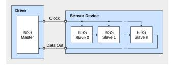
Figure 1: Point-to-point connection: master device connected to single sensor device
