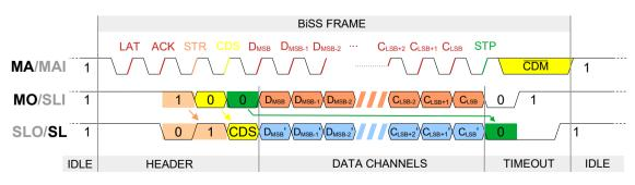
Figure 38: BiSS frame of single actuator bus system
