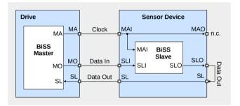
Figure 37: Bus connection with a single actuator slave
