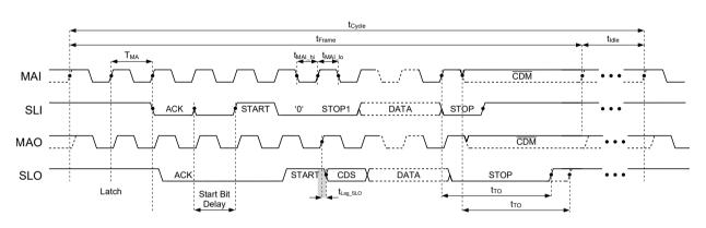
Figure 45: BiSS slave timings for bus configuration
