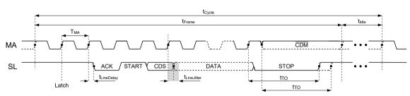
Figure 44: BiSS master timings for point-to-point configuration
