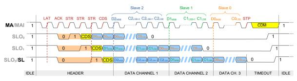
Figure 21: An entire BiSS frame passing through the daisy chain
